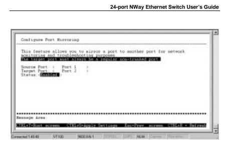
Figure 6-15. Configure Port Mirroring screen
